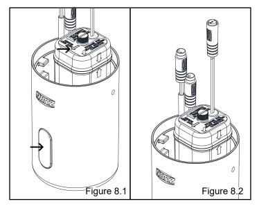
STEP 5A.3 Reattach the sensor cap and tighten cap screws.
