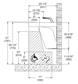
Deck depth must be 20-1/2" minimum for ADA, Enhanced Reach depth is 20-1/2"
