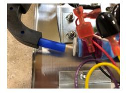
9. Remove two screws holding solenoid from the bracket. Set aside for reuse.
