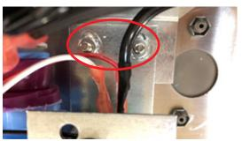
11. Unplug wires from solenoid terminal and remove the solenoid from the aerator connection.
