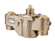
TMV130 MODEL S59-2130 1-1/4" (32.8mm) inlet,1-1/2" (38.1mm) outlet 13 gpm (49.2 lpm) minimum flow capacity
