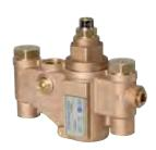
**TMV45 MODEL S59-2045** 3/4" (19mm) inlet, 1" (25.4mm) outlet 5 gpm (18.9 lpm) minimum flow capacity
