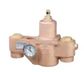
**HL200 MODEL S59-3200** 2" (50.8mm) inlet, 2" (50.8mm) outlet 5 gpm (18.9 lpm) minimum flow capacity
