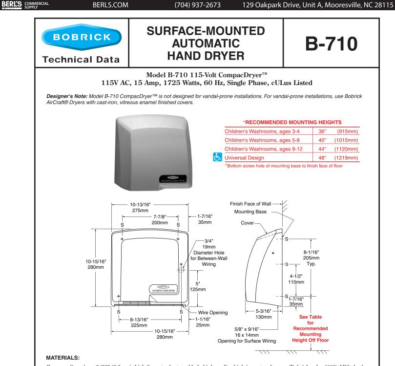
**Cover** — One-piece, 3/32" (2.6mm) thick fire-retardant, molded , high-quality, high-impact, pale grey (Bobrick color #889) ABS plastic, 5-V rated. Cover is secured to mounting base with three flat-head stainless steel screws.
