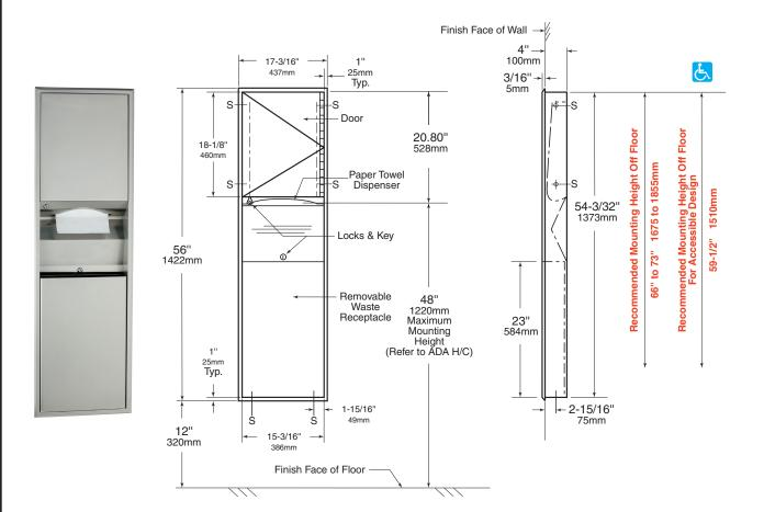
Rough Wall Opening 16" (406mm) wide 54-3/4" (1390mm) high 4" (100mm) minimum recessed depth
